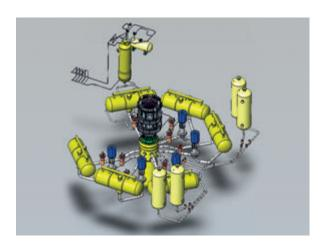
• Laser scanning of selected technology (in cooperation with CSA Systems) and subsequent production of a 3D CAD model of the scanned technology.
